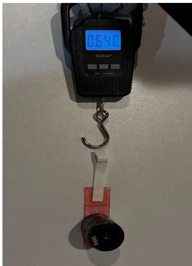
Figure 5.2: Prototype for silicone-coated acrylic samples.
